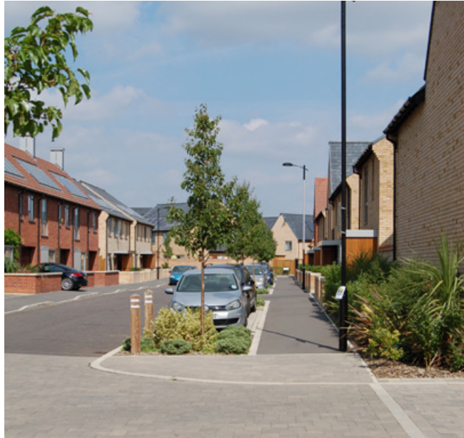
Example of a secondary street with consistent building line and boundary treatment, front gardens, street trees and on street parking.
